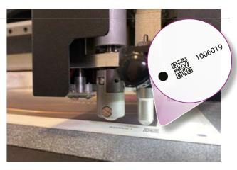
**Colour recognition.** Working with vector lines in the design, it is possible to set-up cutting/creasing processes using different line Colours. This feature recognises different colours and allows users to set types of operation and the processing sequence, by Colour.
